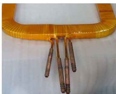
图 3 改进线圈的水冷结构 Fig.3 Improved water cooling structure.
